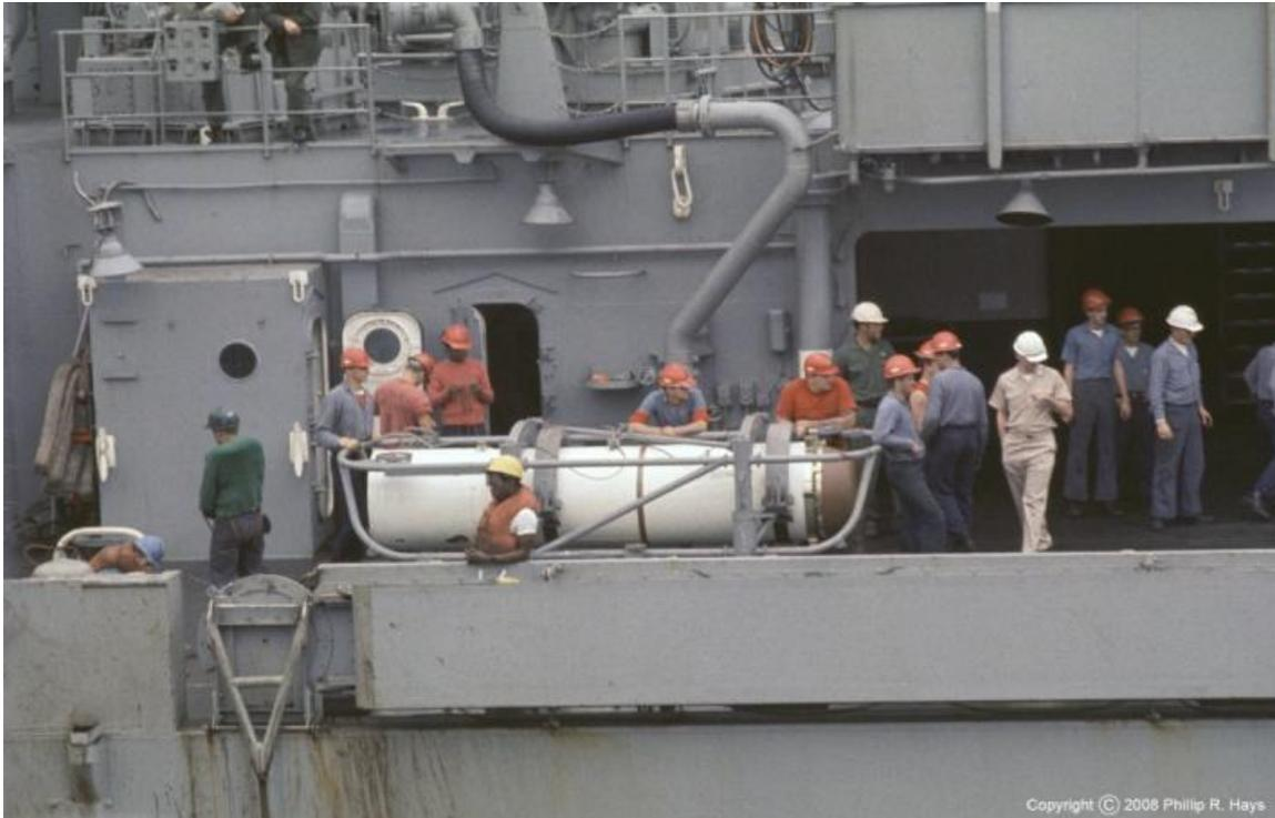
Talos warheads could be transferred independent of the missile. When warheads were shipped they traveled in a special warhead container. Nuclear warheads were always transferred in the can, and never mated to a missile. For security reasons there were no markings on the can to indicate if the enclosed warhead was conventional or nuclear.
