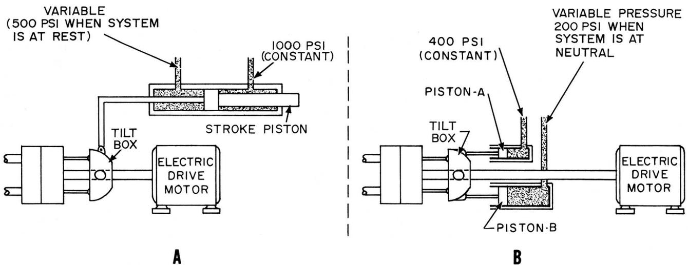
Figure 7-18.— Putting tilt on the A-end: A. Pressure on one piston; B. Pressure applied to two pistons. 83.83
