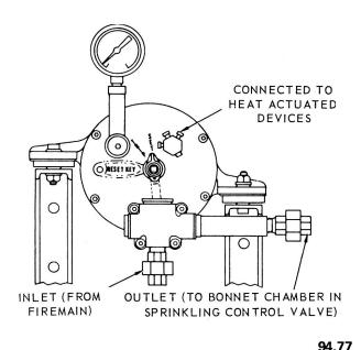
Figure 7-12.—Pneumatically released pilot valve (PRP) used with heat-sensing devices in sprinkler systems.
