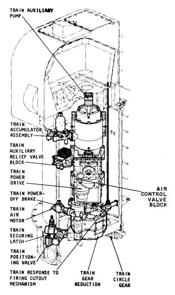
Figure 7-4.—Train system, general arrangement of components.
