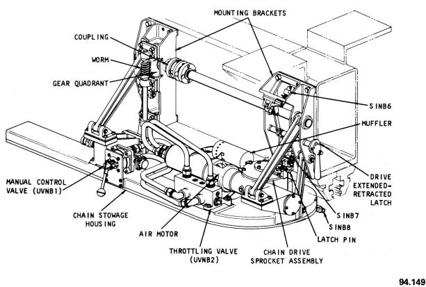
Figure 7-7.--Adapter loading fixture assembly (for Asroc).
