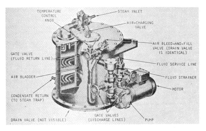
Figure 7-11.—Anti-icing heater tank, Mk 13 launching system (Tartar).
