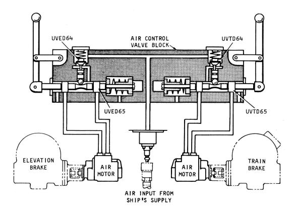
Figure 7-5.—Air control valve assembly.
