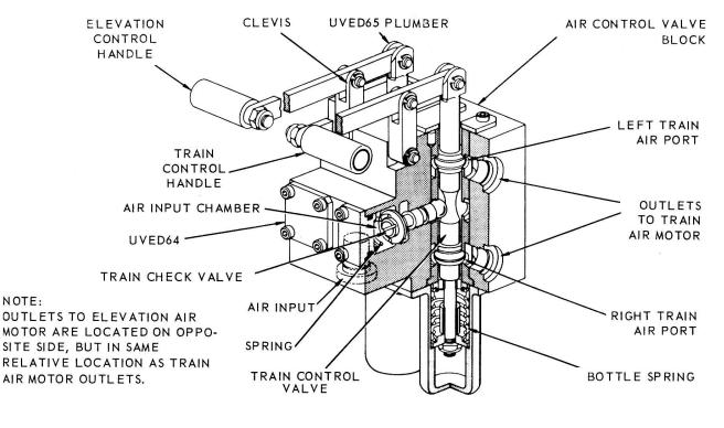
Figure 7-6.—Schematic of air motor drive.
