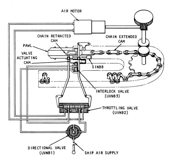
Figure 7-8.—Loading fixture (for Asroc) pneumatic schematic.
