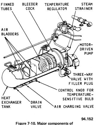
Figure 7-10. Major components of anti-icing system.
