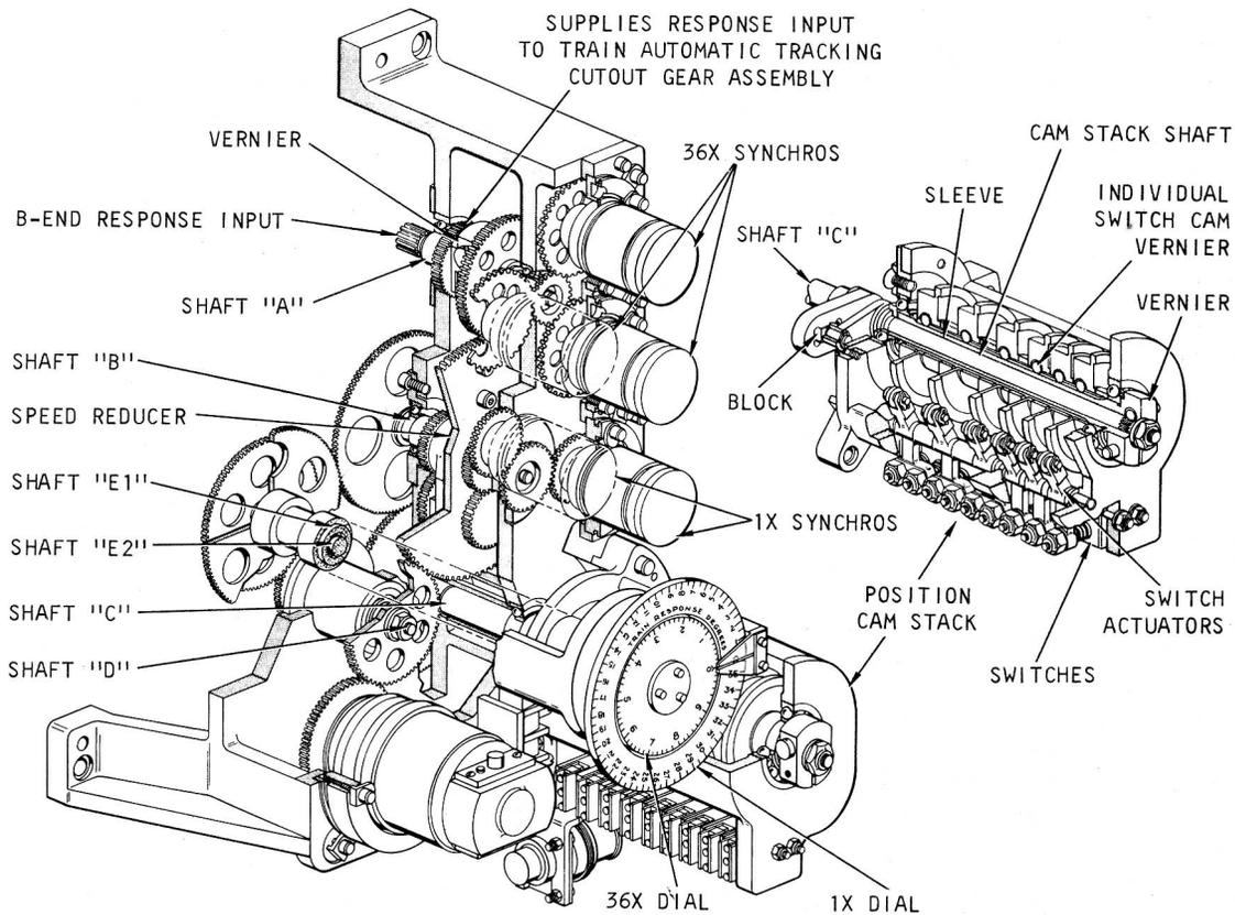
Figure 5-18.—Train synchro gear assembly.
