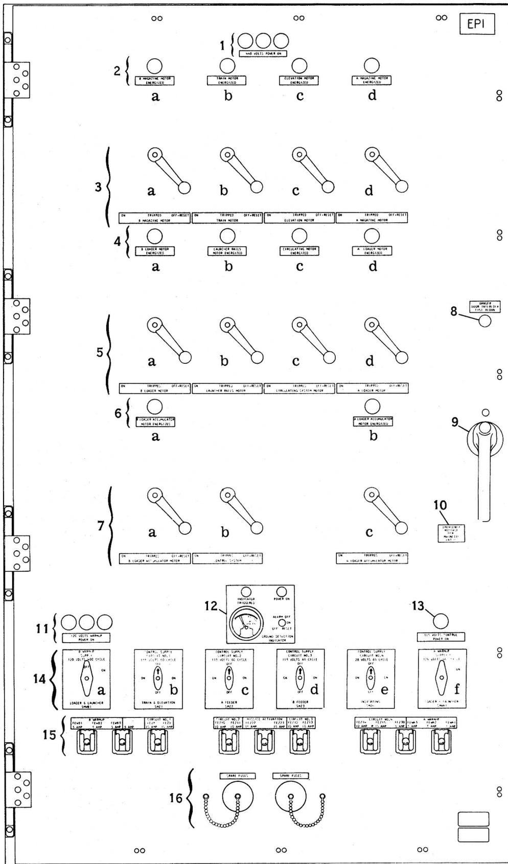
Figure 5-4.—EP 1 panel, Terrier Mk 10 Mod 7 launching system.
