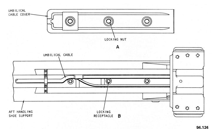
Figure 4-13.–Umbilical cable for Asroc missile: A. Umbilical cable cover; B. Location of umbilical cable on aft handling shoe support.
