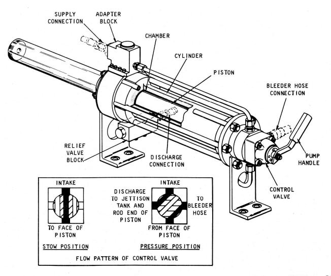
Figure 4-11.-Nitrogen booster pump assembly for jettison device.
