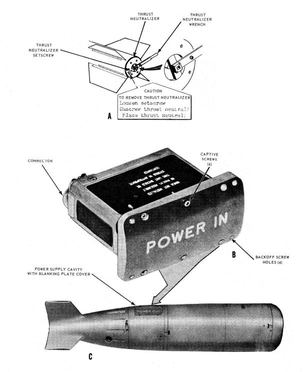
Figure 4-15.—Safing devices restored to Asroc weapon when unloaded: A. Thrust neutralizer; B. Power supply with cover; C. Asroc Depth Charge, showing blanking plate cover placed over power supply cavity.
