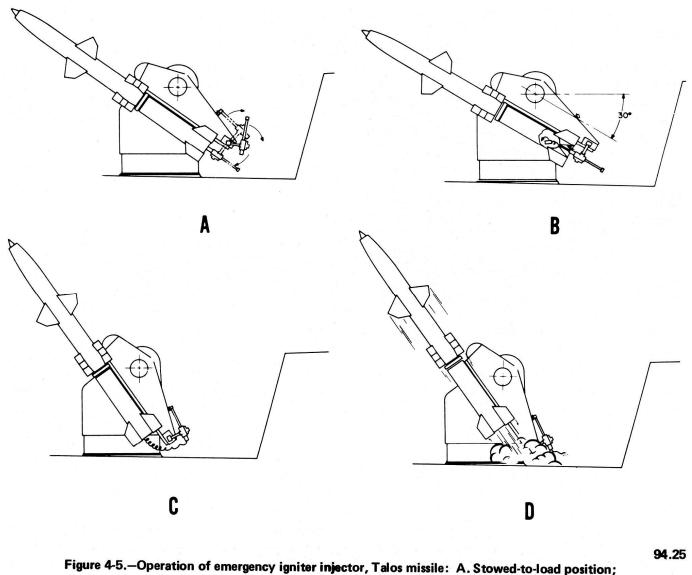
B. Loaded position; C. Firing position; D. Fired.
