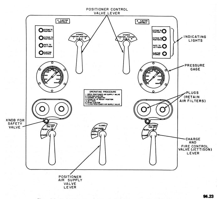
Figure 4-3.-Dud-jettisoning panel, Terrier launching system Mk 10 Mod 0.
