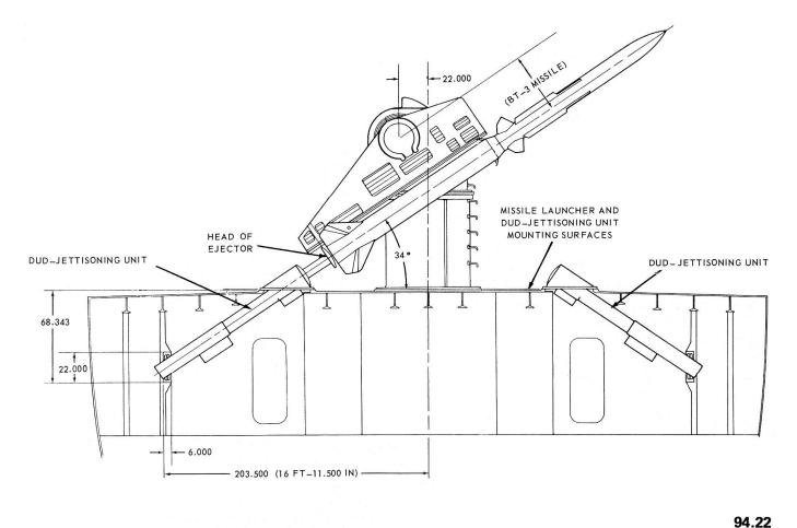
Figure 4-2.-Dud-jettisoning unit Mk 108; cross section view. DLG Terrier installation.
