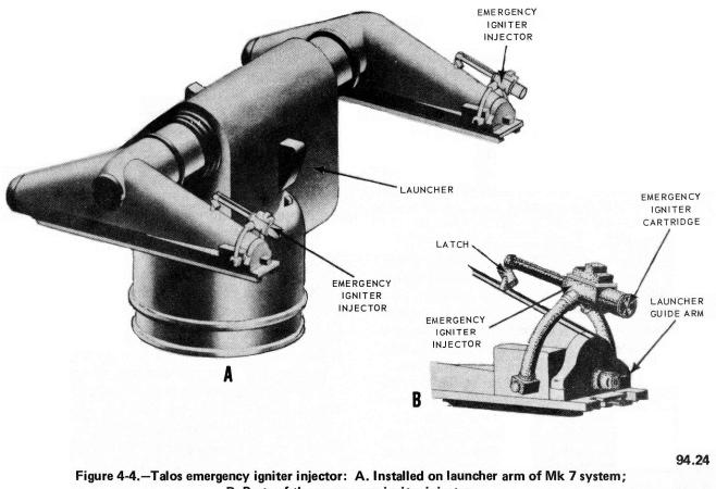
B. Parts of the emergency igniter injector.
