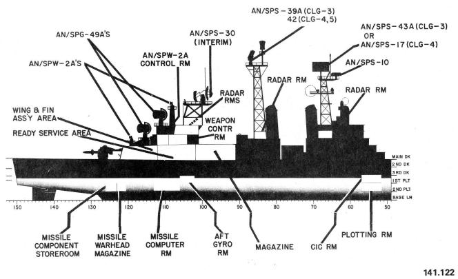
Figure 2-12.-Profile view showing location of missile handling and stowage areas.
