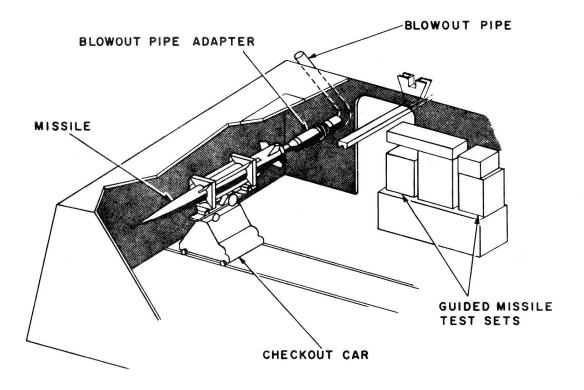
Figure 2-11.-Terrier missile checkout area on a cruiser.
