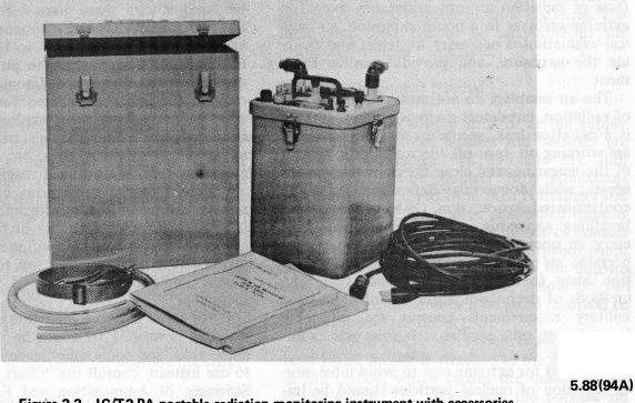
Figure 2-2.-IC/T2-PA portable radiation monitoring instrument with accessories.
