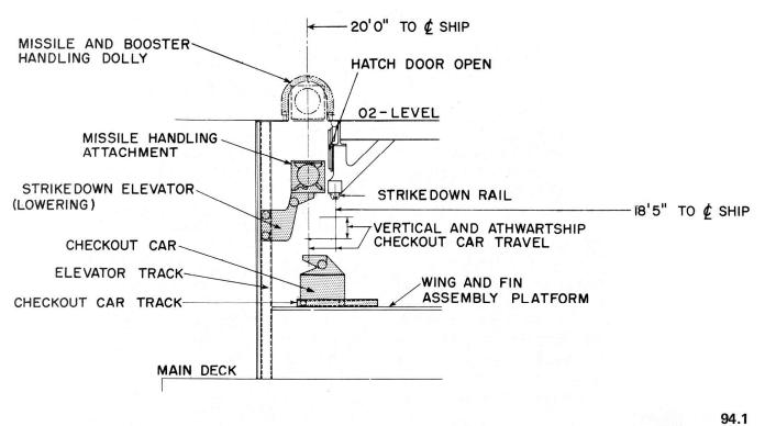
Figure 2-6.-CLG (Terrier). Strikedown and checkout missile handling equipment. (Elevation).
